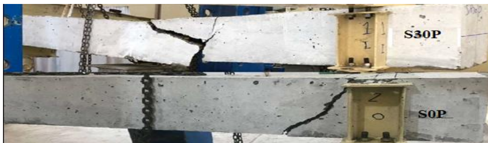
Figure 10. Failure shape of plain concrete beams
