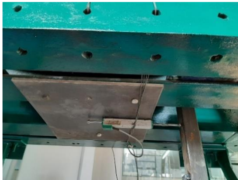
Figure 6. Position of the strain gauge (LVDT) on the shaking table
