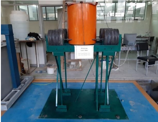
Figure 5. Installation of the structure and the damper on the shaking table
