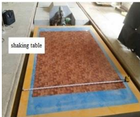
Figure 7. The shaking table used in the experiments
