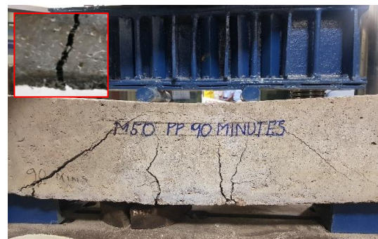
Figure 5. Shear failure of specimen and inset view of crack
