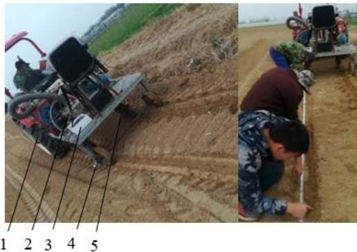
Figure 10. Field test 1. Tractor 2.Waste seed-recycling chamber 3. Control system 4.Encoder 5.SMD
