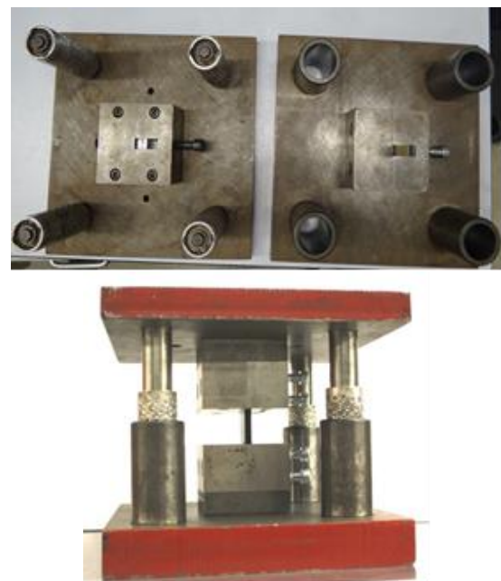
Figure 2. Compressive test fixture with specimen installed
