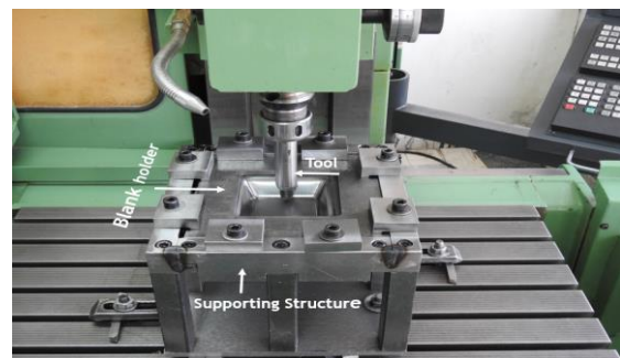
Figure 4. Required equipment for the truncated pyramid SPIF process
