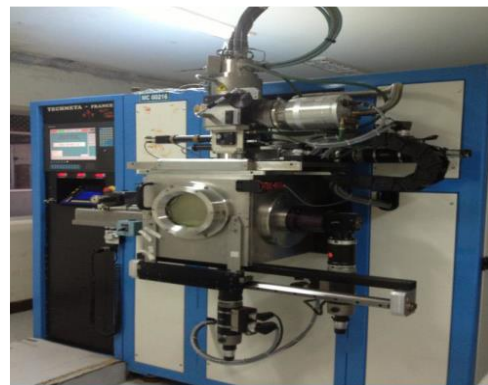
Figure 3. Electron Beam Welding Machine (Techmeta) (courtesy: HAL Korwa)
