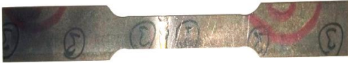
Figure 5. sample fabricated as per standard ASTM E 8/E 8M for Tensile testing
