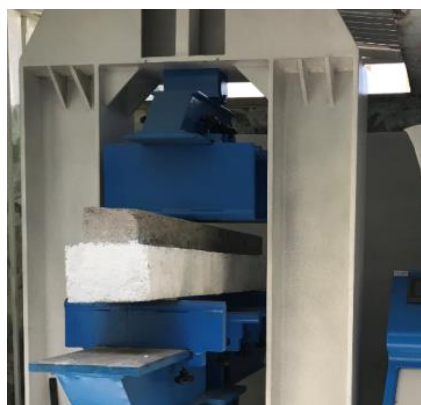
Figure 7. Loading details of the beams
