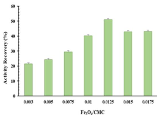
**Figure 6.** Effect of Fe<sub>3</sub>O<sub>4</sub>/CMC Nanoparticles on Activity Recovery of Immobilized Laccase (means of triplicate  $\pm$  standard deviation), pH = 6, Temperature = 4°C, 0.01 g EDC, 0.01 g NHS
