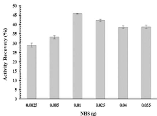
**Figure 5.** Effect of NHS Amount on Activity Recovery of Immobilized Laccase (means of triplicate  $\pm$  standard deviation), pH = 6, Temperature = 4°C, 0.01 g EDC, 0.01 g NPs
