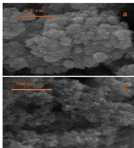
Figure 2. (a) SEM Images of  $\text{Fe}_3\text{O}_4/\text{CMC}$  in 15 kV-200 nm, (b) SEM Images of Immobilized Laccase 15 kV-500 nm
