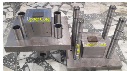
Figure 3. Experimental components of the die set
