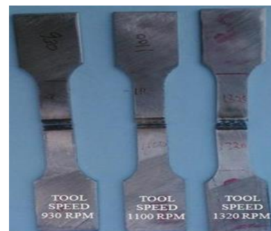
Figure 3. Specimens after tensile testing
