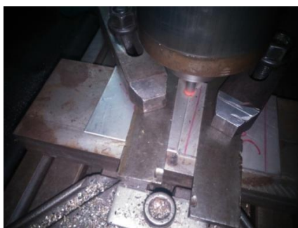
Figure 1. FSW experimental set up
