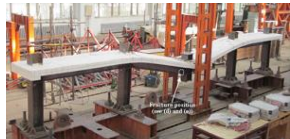
Figure 9. Vertical displacement of the tested frame in the laboratory [27]
