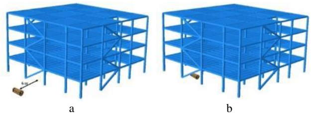
Figure 6. The position of explosive charge a: Outer frame b: Inner frame
