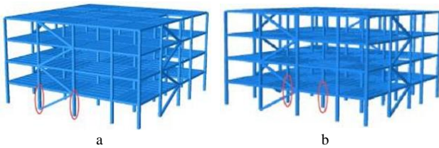
Figure 3. Locations of removed columns in this study (APM) a: Outer frame b: Inner frame
